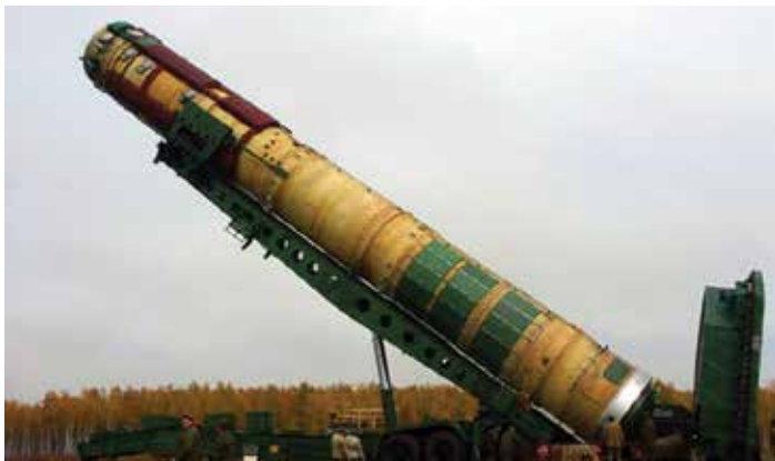
Russia SS-18 Mod 5 ICBM Launch Canister
