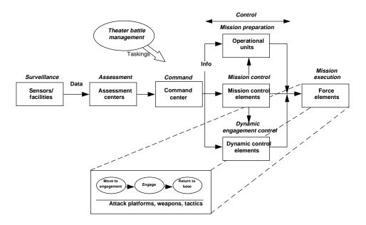
**Figure 8. JFACC Functional Decomposition**<sup>3</sup>
