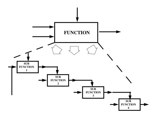
Figure 5. Functional Decomposition of a System<sup>9</sup>
