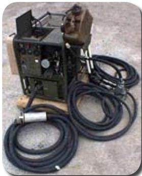
The M17 series Lightweight Decontamination System (LDS) is a portable, lightweight, compact engine driven pump and water heating system. The system is used for operational and thorough decontamination. The LDS is capable of drawing water from any source and delivering it at moderate pressure and controlled temperatures. The system has an accessory kit with hoses, spray wands, and personnel shower hardware. It also includes a collapsible water bladder.
