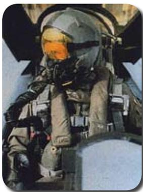
The AERP, MBU-19/P (replaces the MBU-13/P system for aircrews) is a protective mask that enables aircrews to conduct mission operations in a chemical-biological environment. The AERP system includes a protective hood assembly with a standard MBU-12/P mask, an intercom for ground communication, and a blower assembly that provides de-misting. The blower is stowed during flight operations on a bracket that is mounted inside the aircraft.
