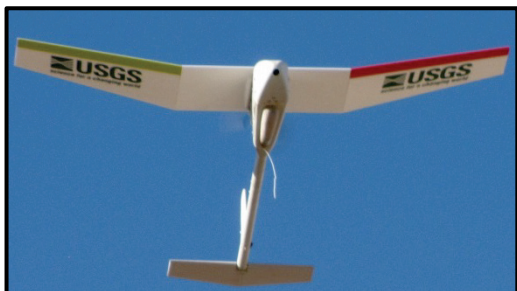
Figure 3. Photograph of a AeroVironment RQ-11A Raven fixed-wing small unmanned aircraft.
