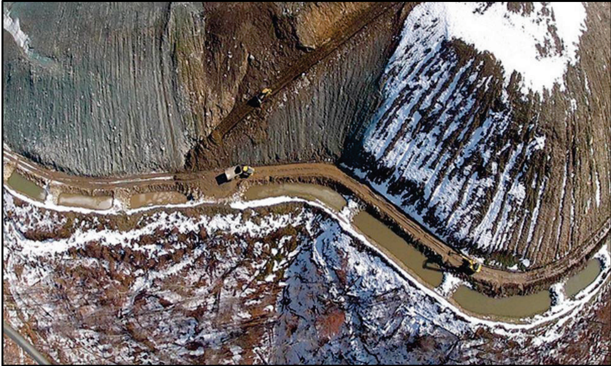
Figure 20. Image of sediment drainage ditches at the Edwight surface mine in West Virginia. Image taken by a GoPro Hero camera on a T-Hawk.
