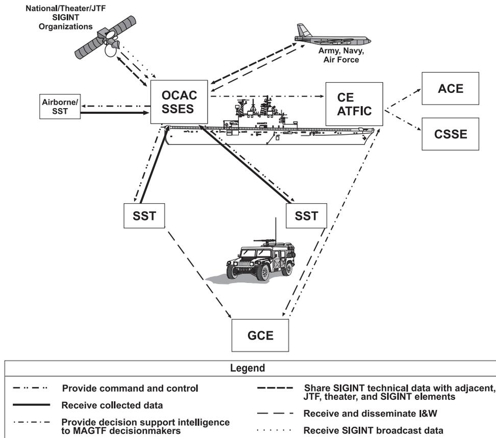
**Figure 6-3. MEU(SOC) CE Afloat SIGINT Operational Architecture.**
