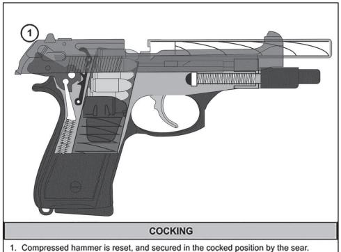
ompressed frammer is reset, and secured in the cocked position by the sear
