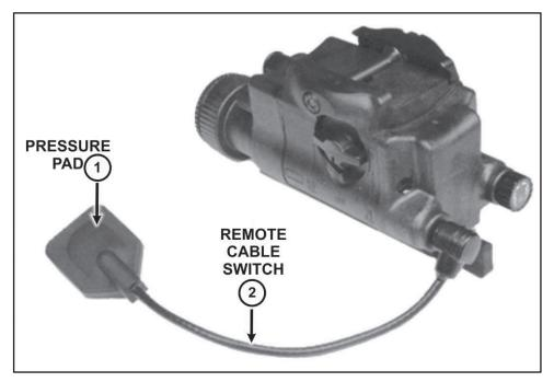
Figure 3-4. Remote cable switch
