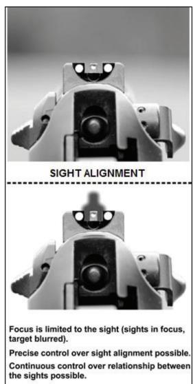
Note: The front sight will be the Soldier's primary focus and it should be seen in clear detail. The target and rear notched sight will be out of focus.
