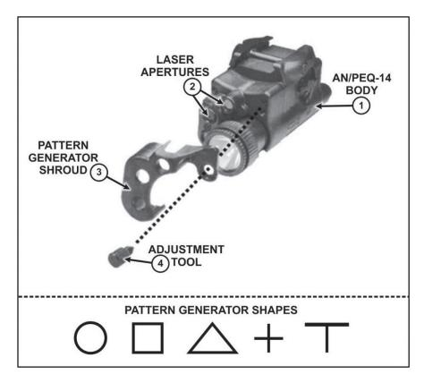
Figure 3-5. Pattern generator install
