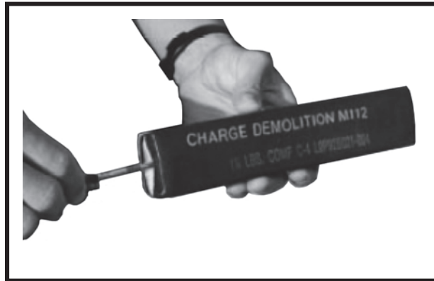
Figure 14-9. Priming of C4 demolition blocks with MDI.
