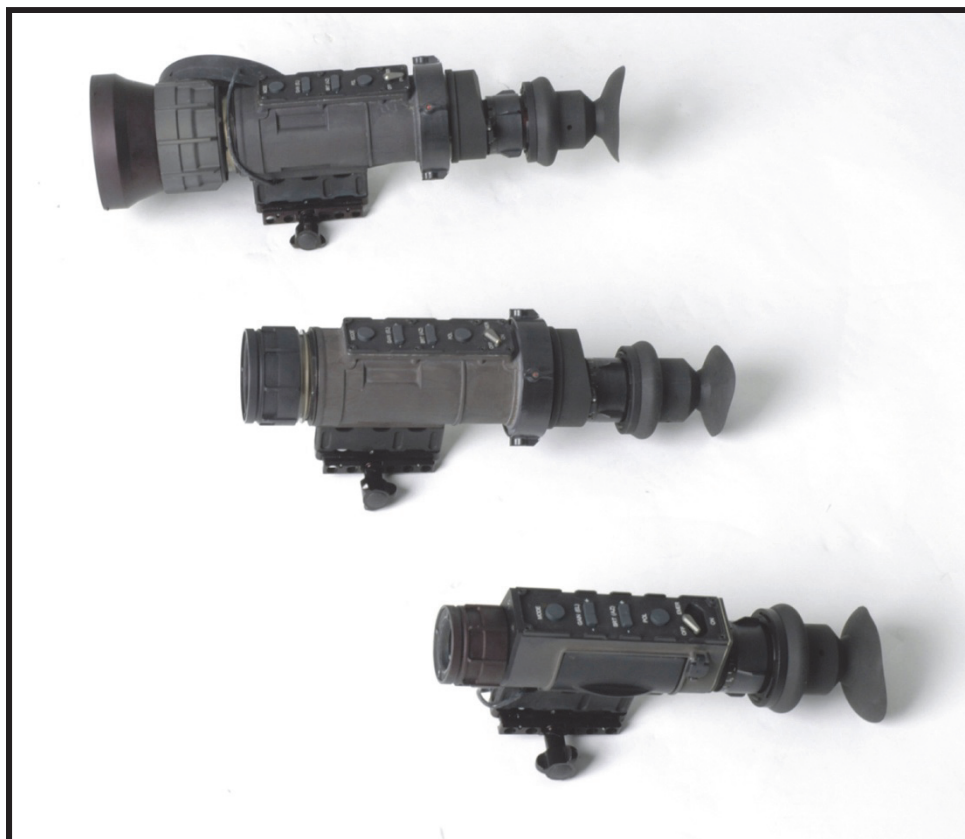
Figure 9-8. AN/PAS-13, V1, V2, and V3.
