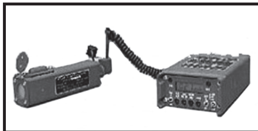
Figure 13-12. Radiac Set AN/VDR 2.
