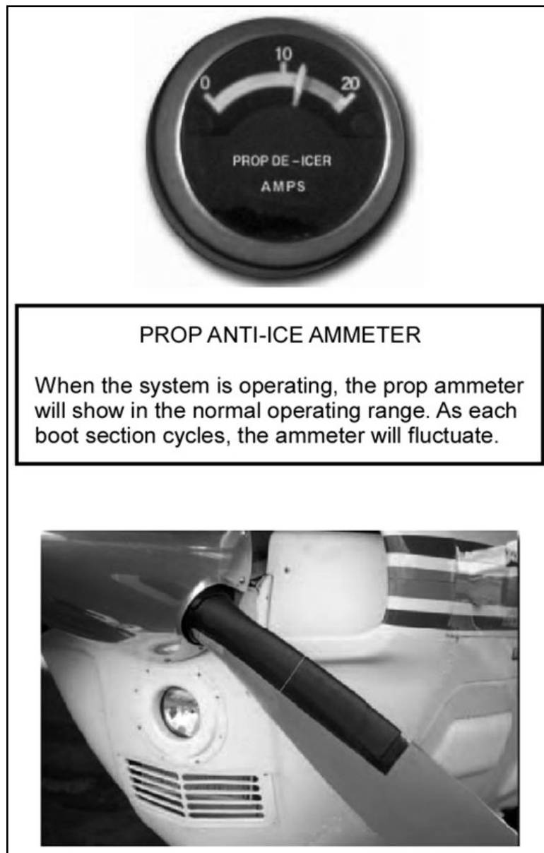
Figure 8-6. Propeller ice control
