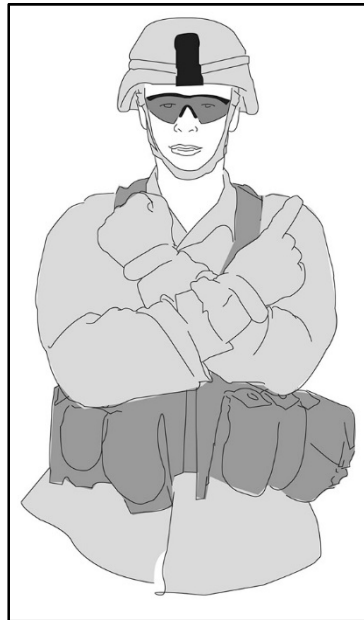
Figure 36. Neutral steer (track vehicles)
