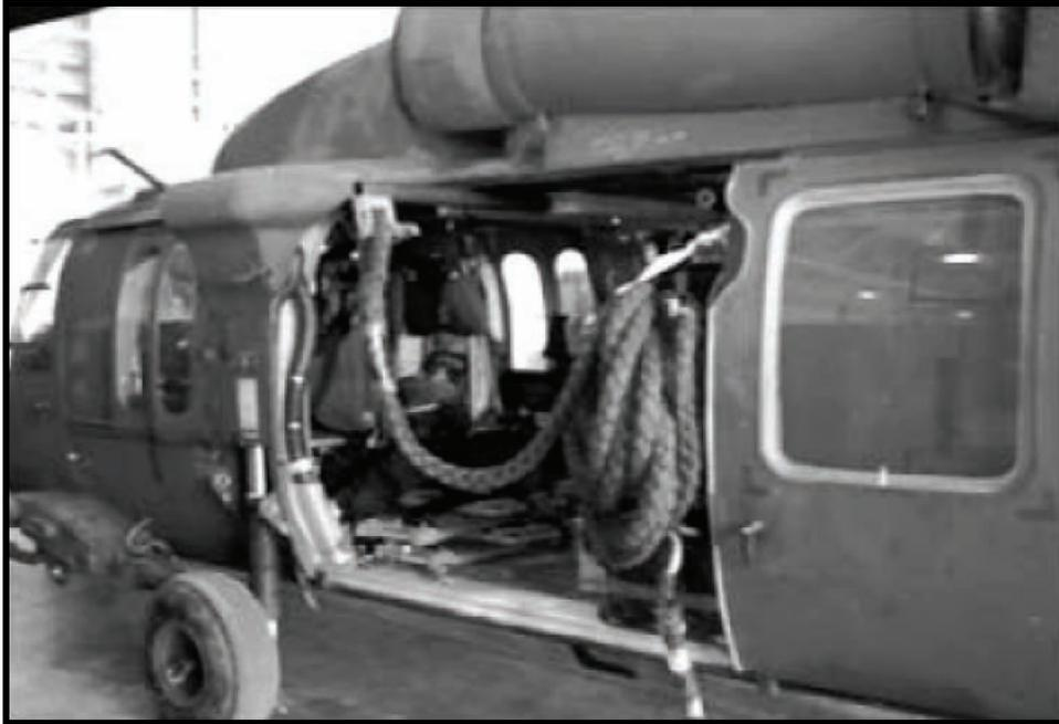
Figure 5-10. UH-60 rigged for fast roping
