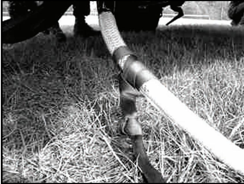
**Figure 5-7. Recovery line with Prusik knot.**
