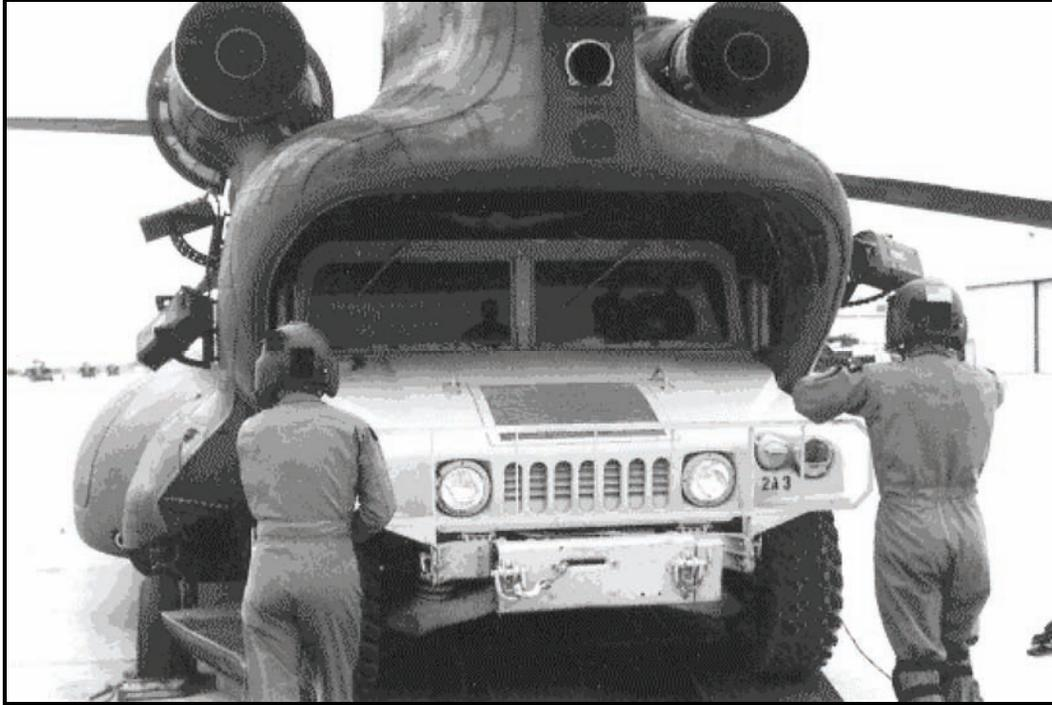
**Figure 5-16. Procedures for loading HMMWV into CH-47 for infiltration.**
