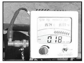
Figure 7-5. Driver's display showing steering directions, distance, and position.
