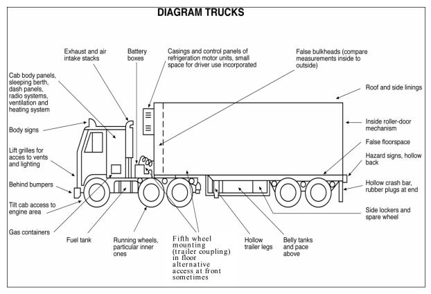
Figure IV-5 Truck Diagram
