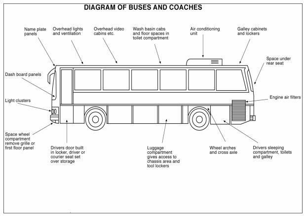
Figure IV-6 Diagram of Buses and Coaches
