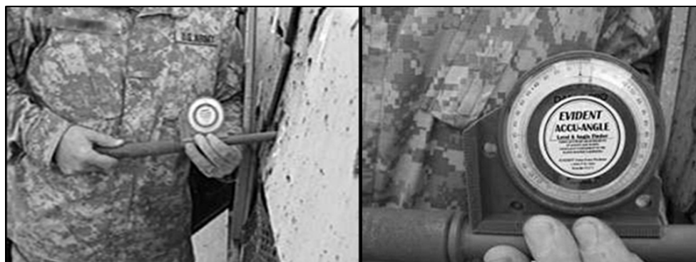
Figure G-38. Using an angle level finder to determine angle of a shot path
