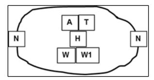
Figure 8-7. Template for area control measure symbols
