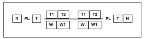
Figure 8-6. Template for line control measure symbols
