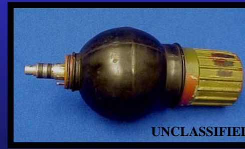
Battery Coolant Unit (BCU)
