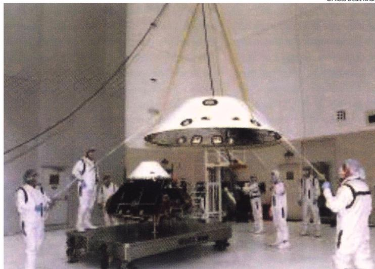
Figure 21. MPL Backshell During Payload Integration<sup>3</sup>
