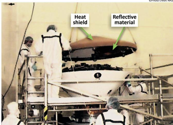
Figure 27. MPL Heat Shield During Payload Integration
