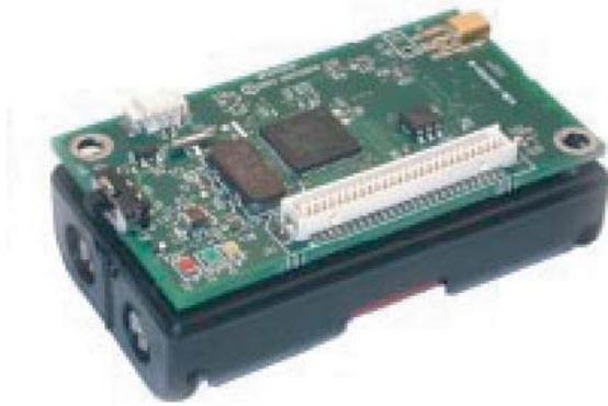
Figure 20: The Crossbow MICA2 wireless node
