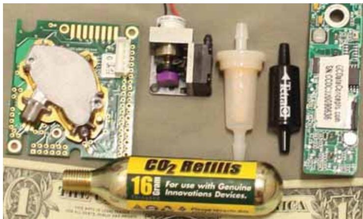
Figure 28: The SenseAir sensor is shown on the left, a small 6V air pump purchased from CO2Meter, a desiccant (white) and CO<sub>2</sub> scrubber (black) we created by filling an aquarium check valve with CaO, our *P* and *T* data-logger from GCDataConcepts is on the right, and a CO<sub>2</sub> cylinder is below. The CaO scrubber can remove the CO<sub>2</sub> from about 500 liters of air and the CO<sub>2</sub> cylinder can fill about 8 liters at STP.
