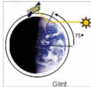
Figure 17: This figure shows the LEO satellite CO<sub>2</sub> monitoring coverage for nadir viewing over land and sun-glint viewing over ocean.
