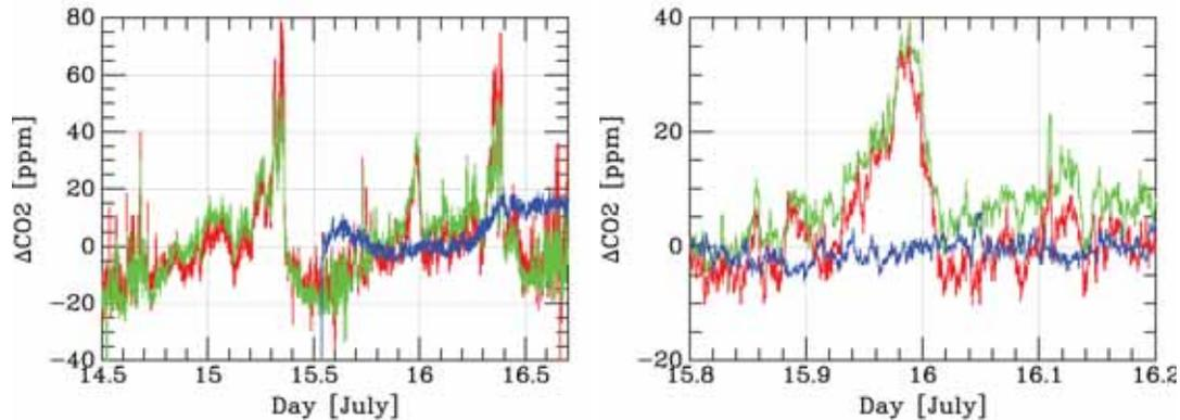
Figure 30: Expanded time history of CO<sub>2</sub> outside Building 29. The three sensors are shown in different colors. The “blue” sensor was placed in a plastic bottle whose slow leakage provided a  $\sim 8$  hour time filter on the CO<sub>2</sub> concentration seen. The RMS variation of the blue samples in the right hand panel is 1.9 ppm.
