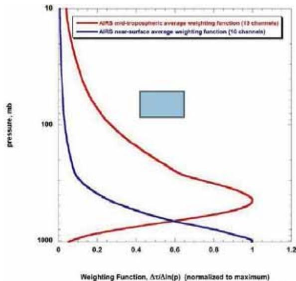
Figure 20: This figure plots the weighting curves that can be used by AIRS to observe CO<sub>2</sub> concentration at various heights in the troposphere.
