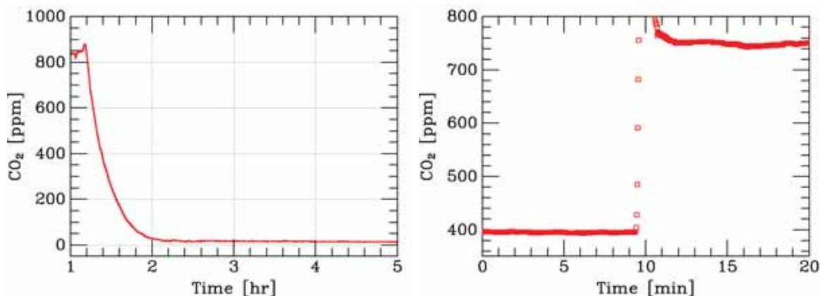
Figure 32: The result of exposing the sensor in a closed bottle with ambient air to a CaO CO<sub>2</sub> scrubber is shown on the left. On the right, a known volume of CO<sub>2</sub> injected into the bottle causes the indicated concentration to rise by  $400 \pm 47$  ppm. The overshoot and subsequent oscillation are artifacts of the dynamic leaky averaging; the RMS prior to injection was 0.9 ppm; the RMS after was 2.8 ppm.
