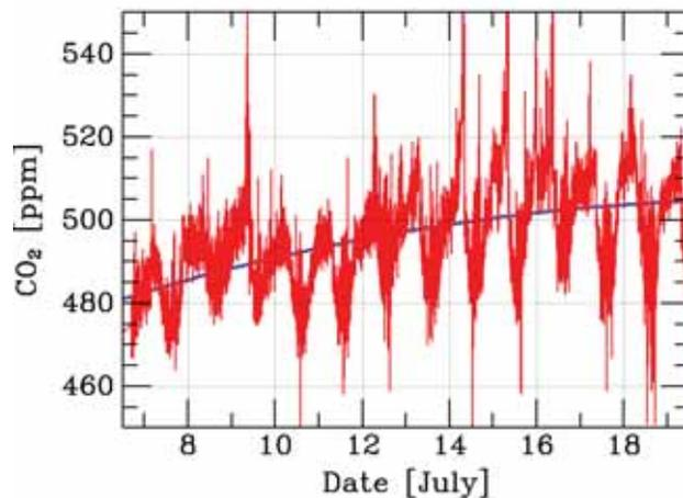
Figure 29: Two weeks of CO<sub>2</sub> concentration outside Building 29 is shown for one of the sensors. The drift indicated by the blue line is probably a sensor artifact; the shorter term variation is real. July 10, 11, and 17,18 were weekends.
