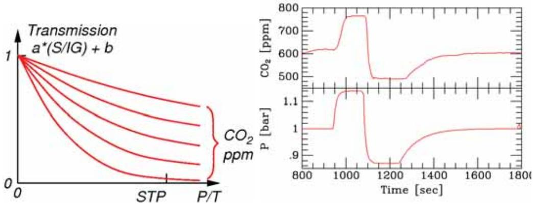
Figure 31: A notional graph showing the effect on transmission through a fixed gas cell on CO<sub>2</sub> density (proportional to  $P/T$ ) and on CO<sub>2</sub> concentration is shown on the left. The transmission should be proportional to the measured signal  $S$  divided by the light intensity  $I$  and system gain  $G$ , with some offset and scale to be determined. The effects we observed by varying  $P$  are shown on the right.
