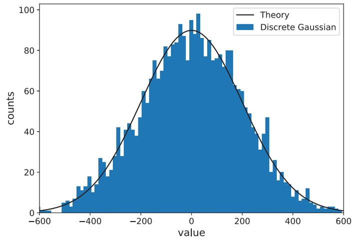
Figure 6-4: Histogram of the sampled discrete Gaussian noise added to the population query. The standard deviation of the parent distribution is 200. The solid line represents the theoretical continuous Gaussian distribution.
