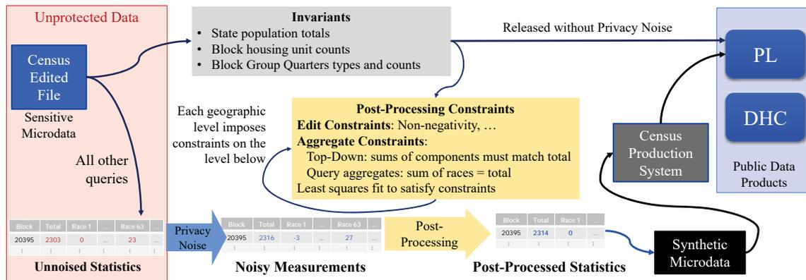
Figure 5-1: Process used to produce privacy-protected data products.
