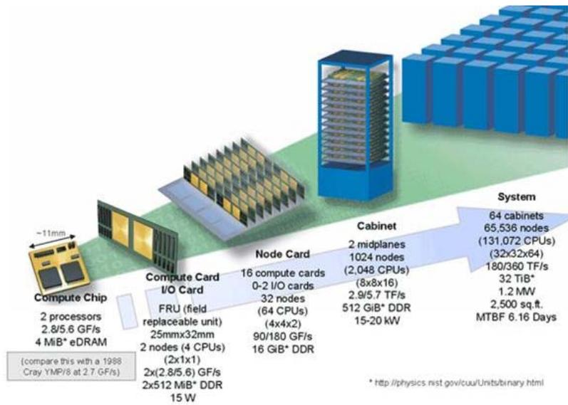
Figure 2-2: Hardware design schematic for IBM's Blue Gene/L.
