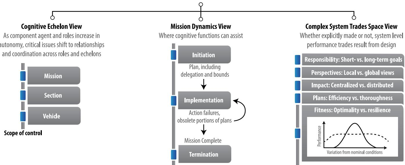
An autonomous system reference framework highlights the allocation of cognitive functions between the human operator and the computer. *The Role of Autonomy in the DoD Systems* (2012).
