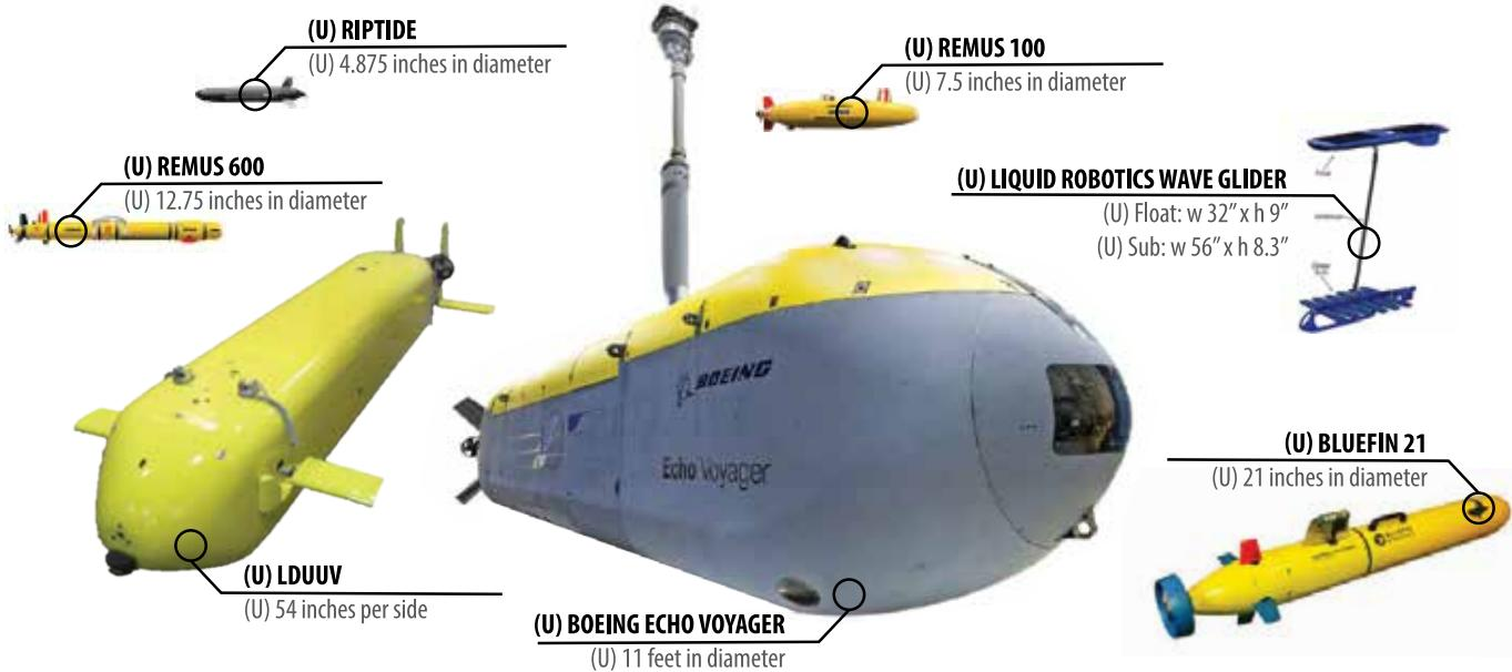
Several commercial unmanned undersea vehicles have been adapted for military use at a far lower cost than a traditional DOD acquisition program, as described in *Next Generation Unmanned Undersea Systems (final report in progress)*.
