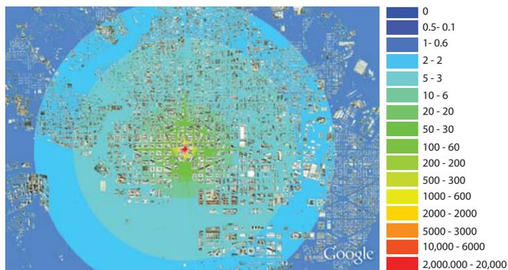
Figure A-9. Ground overpressures in psi modeled by NucFast for the illustrative Washington, DC scenario.
