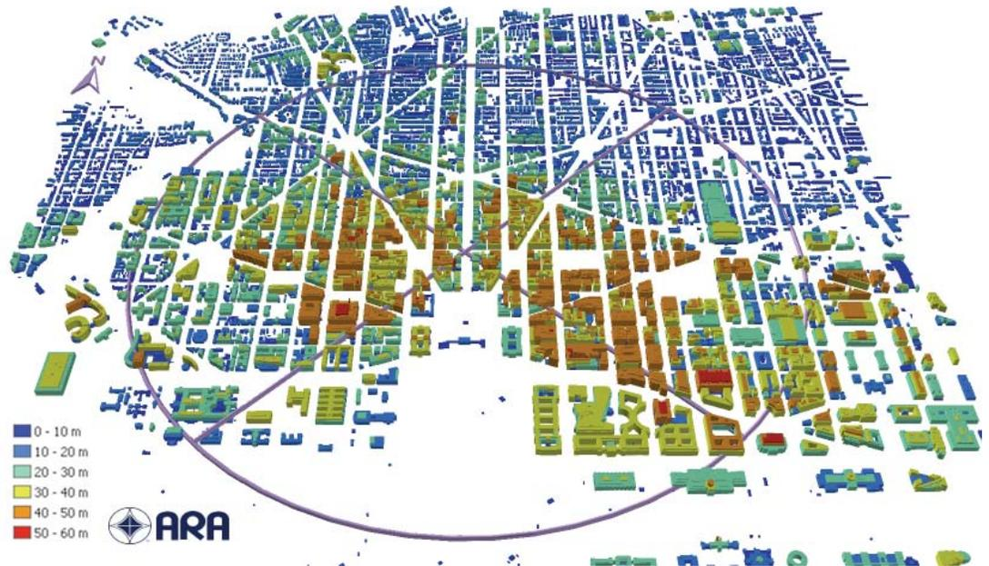
mitigating effects an urban environment might have, researchers at ARA modeled structures in the Washington, DC environment and calculated the effect on prompt radiation fields. Figure A-14 is an image of the “virtual city” that was modeled to calculate how the prompt radiation field might be affected by an urban environment.
