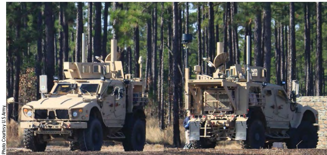
A pair of Prophet Enhanced system trucks sit in a training area during a recent field training exercise. The Prophet system has sensors that can intercept enemy radio communications and radio frequencies, and allows the Soldiers manning the trucks to conduct analysis.
