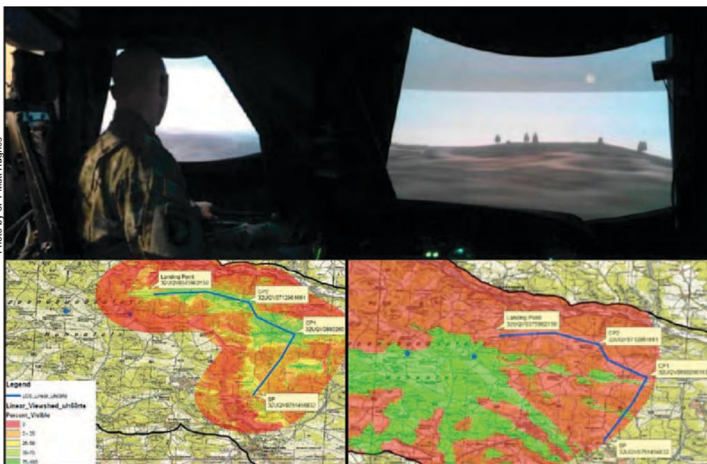
(Clockwise) In November 2015, CW2 Deuel flew the UH-60 flight simulator at Illesheim, Germany along a route he templated for HTA, Germany using SAGE. He modeled air ambush teams' radial line-of-sight and generated a linear viewshed along his flight path to determine visual detection probability along the route.
