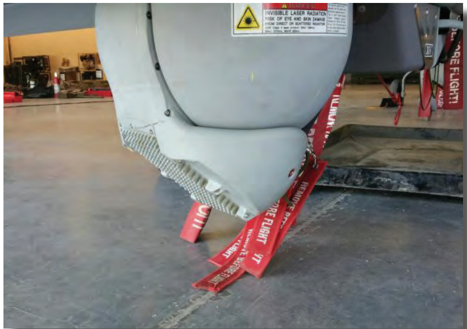
Approximately 2 inches from the ground, the Shadow's IR laser designator as it appears on a RQ-7B.
