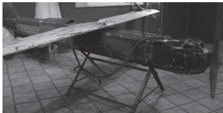
SD-1 Surveillance Drone was a radio controlled plane used from 1957 to 1961 primarily for photo surveillance.
