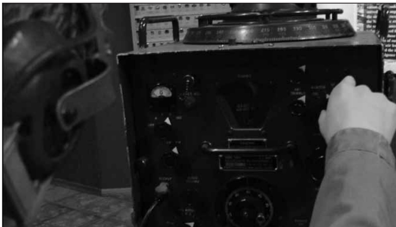
AN/PRD-1 direction finding set determined what direction enemy radio signals were coming from.
