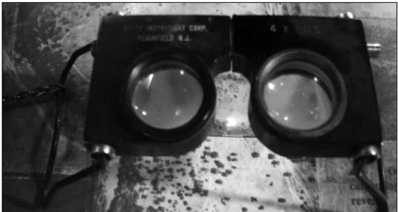
The Lens Stereoscope provided a three dimensional view of an image. It was low cost, compact, and portable
