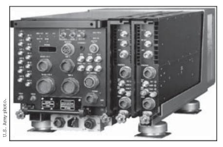
The Joint Tactical Terminal can provide a transmit capability and an eightchannel receive capability. The terminal receives intelligence broadcasts from TOPS, TDDS, TIBS, and TRIXS.<sup>1</sup> It can also receive imagery from imagery product libraries.
