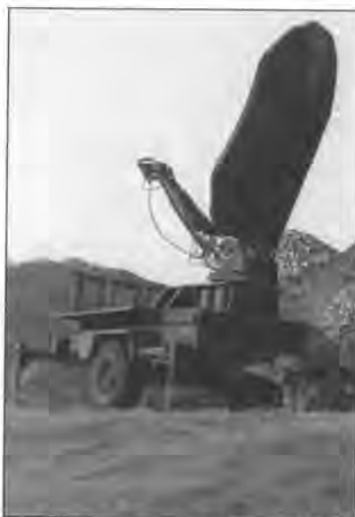
TROJAN SPIRIT II provides worldwide secure voice, data, facsimile, video, and secondary imagery dissemination capabilities.
